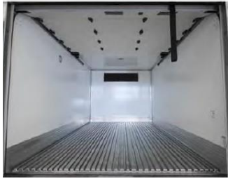
Image 5: Trailers without side-board and no mechanism to lock cargo bars
