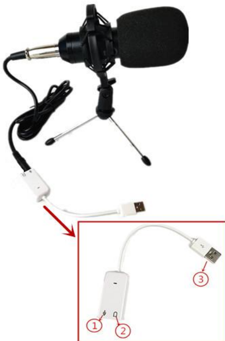
NO.5: As shown, Figure ① connects the microphone; Figure ② connects the earphone or other applicable speakers;
