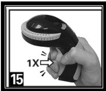
Firmly squeeze the handle to cut the tape.
