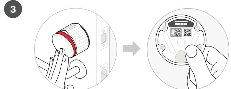
You will then need to scan the QR Code for your smart lock. Push inward on the 'a' to remove the battery cover and flip it over to reveal your code.
