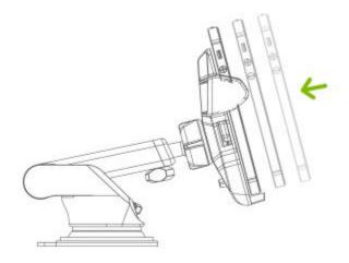
5. Place your device inside the mount firmly to activate the one touch locking system.
