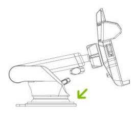
2. Place the suction pad on desired surface & press down.
