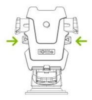
4. Press side buttons into locking position.
