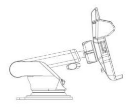
8. Tighten knob to fasten in place.
