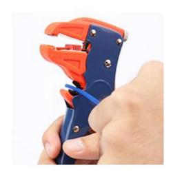
2. Grasp the handle firmly and cut the wire
