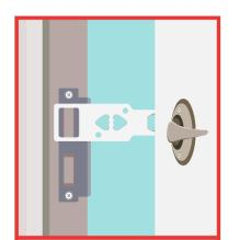
Insert the metal piece into the strike of the door
