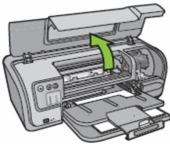
3. Wait until the carriage moves to the right side of the printer and is idle and quiet.
