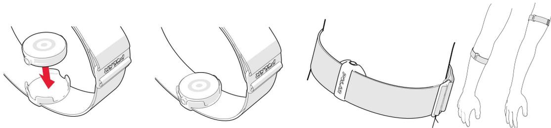
The sensor must be in firm skin contact, but not too tight to prevent blood flow. For most accurate heart rate measurement, we advise you to wear your OH1 for a few minutes prior to starting the heart rate measurement.
