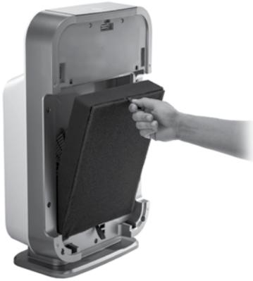
3. Remove the used filter by pulling out on the pull strings. Place the used filter in a plastic bag to prevent dust from re-entering the air.
