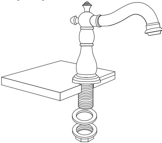
4. Remove the lock nut, metal washer, and rubber gasket from the handle valve labeled 'cold.' Insert the handle valve into the faucet hole on the right.
