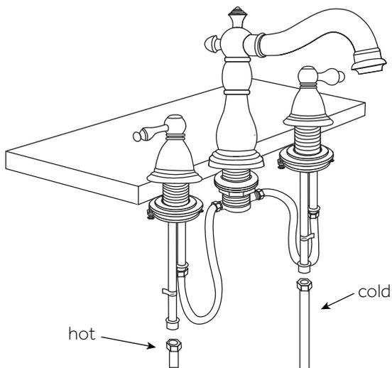
9. Once installation is complete, turn the main water supply back on from underneath your sink. Check for any leaks underneath.
