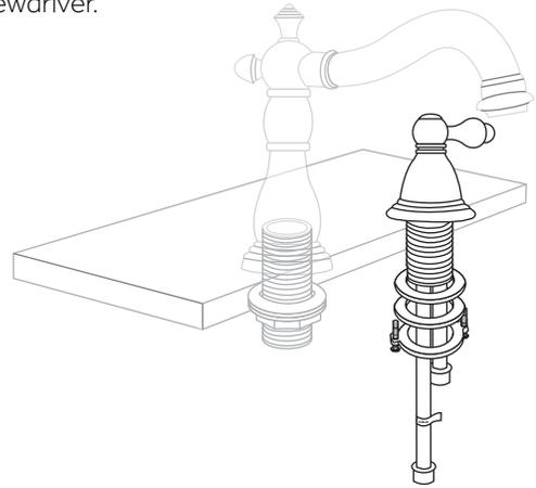
6. Repeat steps 4 and 5 for installing the 'hot' handle valve into the left faucet hole.
