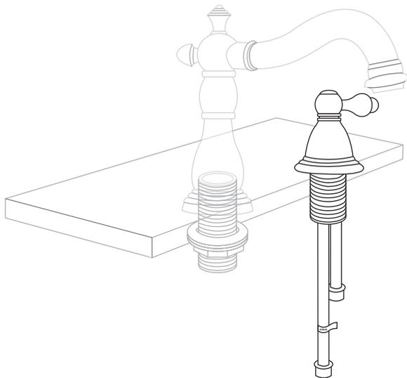
5. From under the counter, slide the rubber gasket back onto the handle valve followed by the metal washer. Secure the handle valve to the counter by hand tightening the lock nut. Finish securing by tightening the screws on the lock nut using a Philips head screwdriver.
