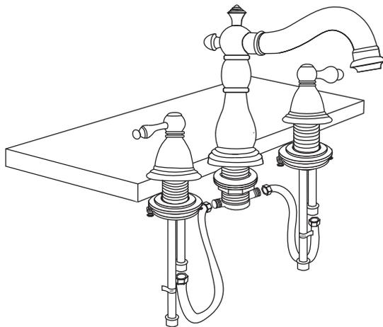
8. Attach the main water lines to the proper inlet of each handle valve. Use an adjustable wrench to tighten, but be careful not to overtighten. Apply thread sealant or plumber's tape to each threaded connection. Ensure that you are connecting the hot and cold lines appropriately.
