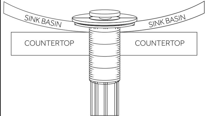
5. From under your counter, slide the tapered rubber gasket followed by the plastic friction washer onto the tailpiece until they meet your sink or countertop. Be sure that the tapered side of the rubber washer is facing up.
