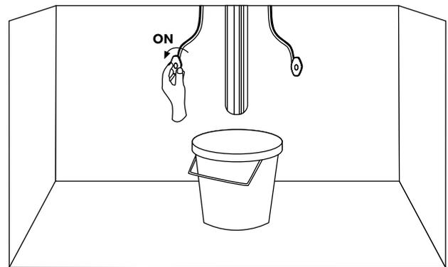
10. Remove the aerator from the spout and turn the faucet on for approximately 60 seconds to allow any dust or loose sediment to exit the water lines. Check for any leaks. Test both hot and cold water to ensure they are running properly. Once complete, reattach the aerator.
