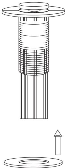
4. Insert the drain flange and tailpiece through the top of your sink's drain hole.
