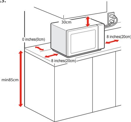
A minimum clearance of 8 inches (20cm) is required between the oven and any adjacent walls.
