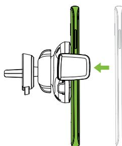
**4** - Put smartphone against the Easy One Touch Trigger Button, arms will automatically close against the device
