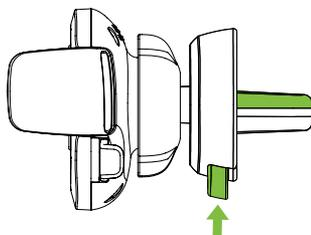
**2** - Press the Lock & Release button to attach to vent
