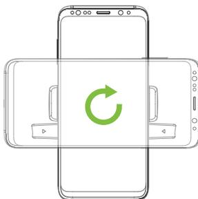
**7** - Rotate Cradle into Landscape mode. Tighten to lock in desired position.
