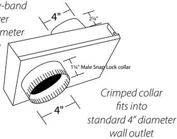
Functional length 5" from center of dryer outlet to center of wall outlet
