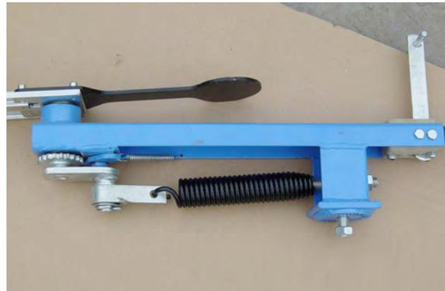
Rotate the arm counter clockwise into the 1 o'clock position. Hook the black main spring into the silver swiveling spring hook, which is attached underneath the throwing arm/clutch pivot point.
