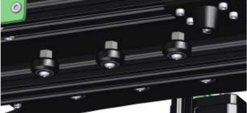
2. Adjust the tension of the gantry wheels on the right pillar of the gantry frame.
