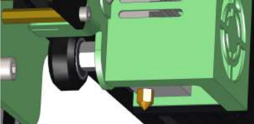
4. Check the tension of the belt driving the Y-axis (under the build plate). The belt should be taut, with no slack or slop.
