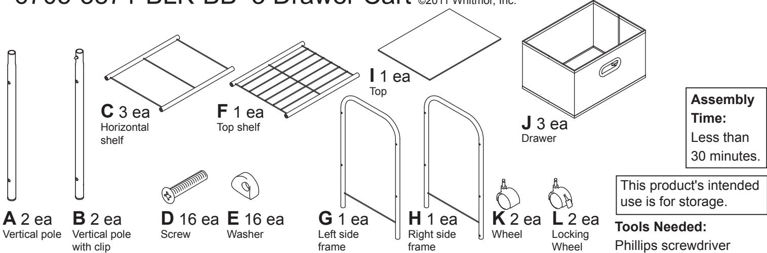
**STEP 1.** Starting with the bottom section, attach vertical poles (A & B) to two horizontal shelves (C) using screws (D) and placing washers (E) between poles and shelf.
