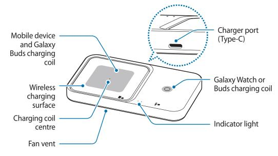
The Wireless charger can charge one device on the mobile device and Galaxy Buds charging coil and watch or buds charging coil.
