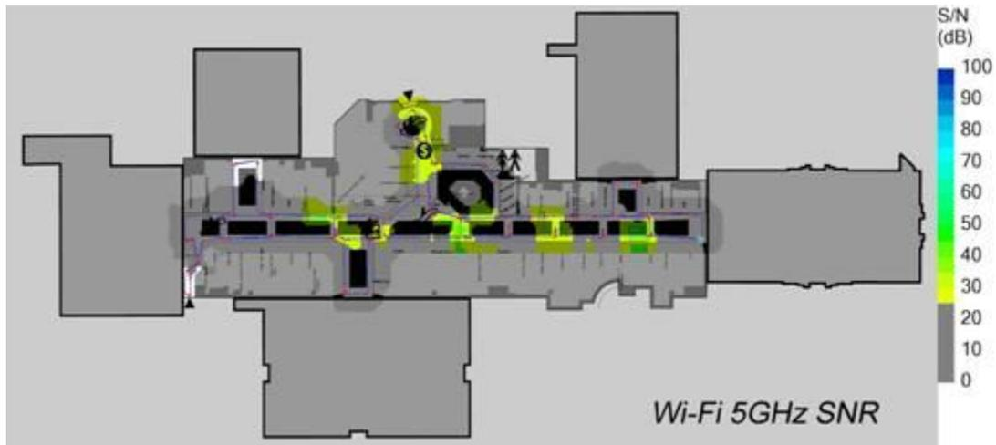
*SNR: Signal-to-noise ratio is a measure used in science and engineering that compares the level of a desired Signal to the level of background Noise. It is defined as the ratio of signal power to the noise power. A ratio higher than 1:1 (or 0dB) indicates more signal than noise.*
