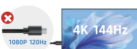
Cable specs mismatch (e.g. 1080P/120Hz cable to 4K/144Hz monitor)
