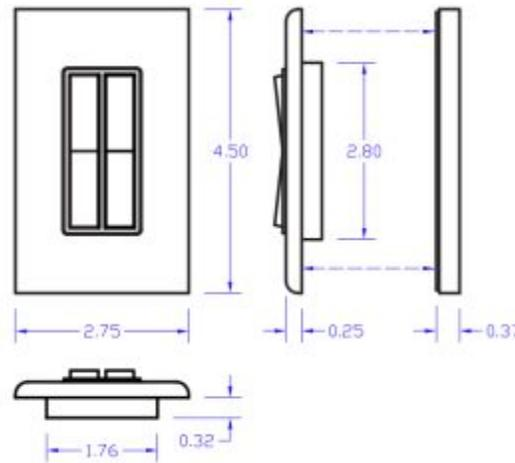
The light switch is compatible with standard decorator style faceplates. A screwless faceplate is included.
