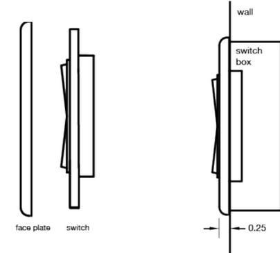
**Option B:** Surface mount backplate to a flat surface using included Command Strips or with screws (not included). If using Command Strips, make pull tabs accessible from center of backplate. After the backplate is mounted, attach switch to backplate using included  $\frac{3}{8}$ " backplate attachment screws. Snap on screwless faceplate.
