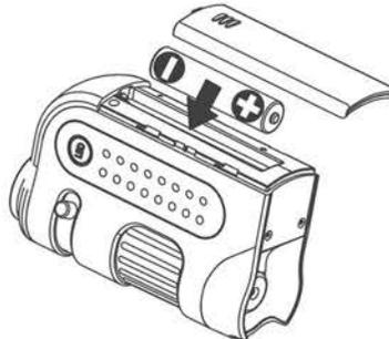
3. Attach the battery door ① as shown below.
