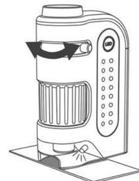
4. Rotate the focusing ring ⑥ until the image is sharp and clear.
