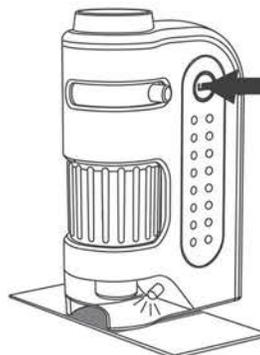
3. Adjust the zooming dial ④ to the desired level of magnification.
