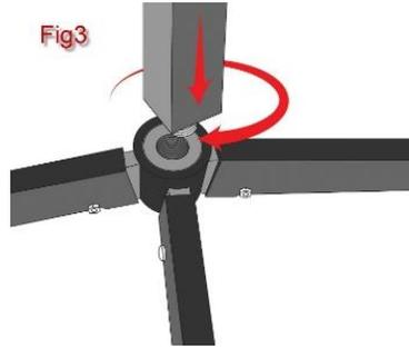
**Step 3** – Take the chrome center piece (I) that goes in the main post, pull the locking pin (J) and insert the chrome center piece. Make sure that the holes in the chrome post align with the locking pin, turn the locking pin (you will hear a click sound) to lock it in place. For additional security of the product tighten the knob (J) on the main post (see Figure 4).
