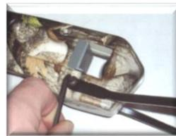
3. Insert the steel pressure plate into the “U” shaped grey nylon front limb protector.
