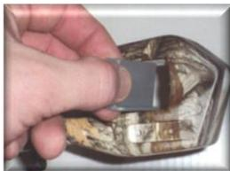
2. Install the foot stirrup using the 2 screws included in the hardware packet. Tighten securely on both sides.
