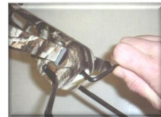
6. Install the limb tip covers on both ends of the limb. Push on by hand until secure and tap on a solid surface to seat ALL the way on to avoid damage when stringing.
