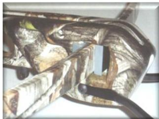
5. Align the limb so the 2 vertical indicators printed on the limb are centered on either side of the opening. Hand tighten the nose bolt and be sure the limb remains centered. Tighten the nose bolt with the supplied Allen key wrench securely.
