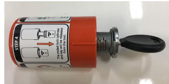
**STEP 5:** Remove cap from tumbler shell, then install tumbler assembly with key.
