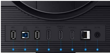
USB Type-A Downstream USB Type-B Upstream USB Type-A Downstream DP IN HDMI IN 1 HDMI IN 2 LAN POWER
