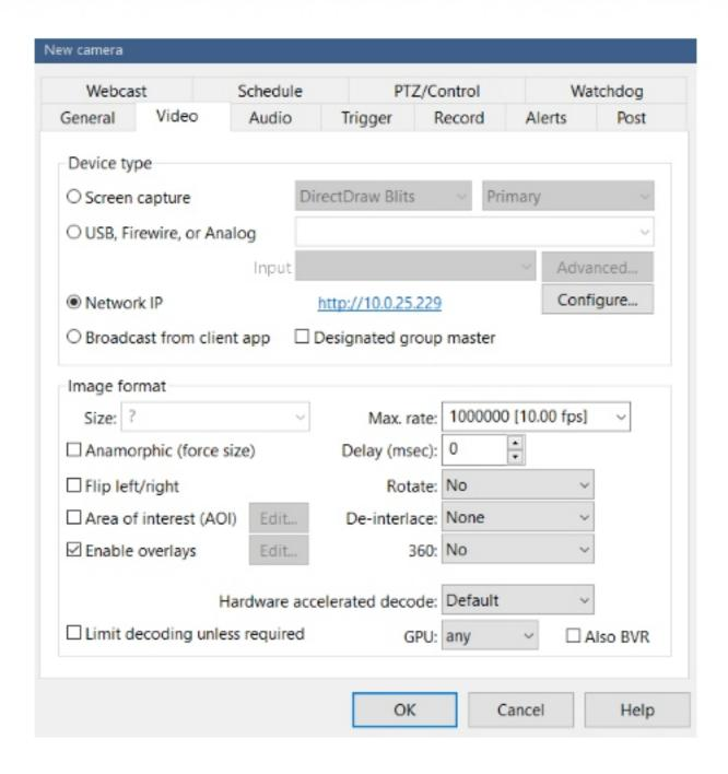
The page is defaulted to the Video tab. The options available for adjustment are Image Format and Frame Rate, PTZ Controls, Recording through Blue Iris, Alerts through Blue Iris, and other features. Once you have finished adjusting any necessary settings, click on OK to add the camera. The live view screen of your camera will show in the interface.
