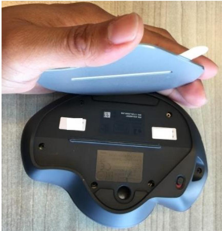
2. Eject the ball with the back of a pen, through the hole on the bottom.
