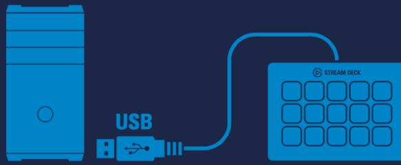
Connect **Stream Deck** directly to a USB port on your PC or Mac – do not use a USB hub.
