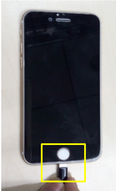
OK: plugging vertically
