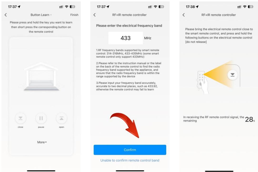
Suppose you choose the garage door, and its remote control is 433 band, Please enter 433 in the frequency band, Point the handheld remote control at the universal remote control, Hold down one of the function keys for 3 seconds.
