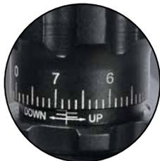
2. There are horizontal and vertical hash marks beneath the elevation and windage turret that are easy to see and indicate how many rotations you have dialed in after making adjustments beyond your zero. The bottom edge of the turret will reveal a hash mark each time you have made  $\frac{1}{2}$  a rotation when moving up in elevation or to the right in windage and vice versa.
