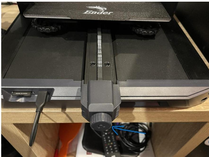
1. Loosen the Y belt tensioner on the front of the machine so that there is slack in the belt.
