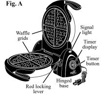
the display time rapidly until you have reached the desired time. The timer can be set for 1 to 30 minutes. The timer will automatically begin counting down approximately two seconds after it is set. To reset the timer to zero, press and hold the timer button for about two seconds.
