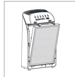
Remove any packing from the new filter element and take notice of the inward and outward sides of the filter element.
