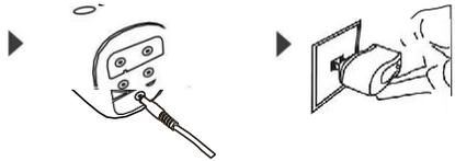
4. Insert two air hose plugs into the controller correctly and completely.
