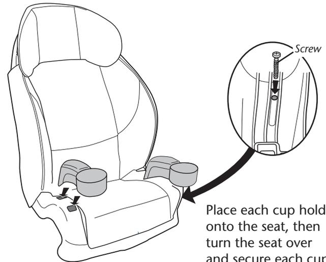
Place each cup holder onto the seat, then turn the seat over and secure each cup
