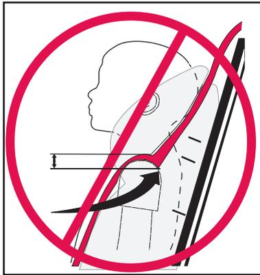
If the child's shoulders are high enough that routing the shoulder belt under the head rest causes the belt to be pulled down the back side of the child's shoulder (before passing through the head rest), the belt should not be routed between the seat and the headrest.
