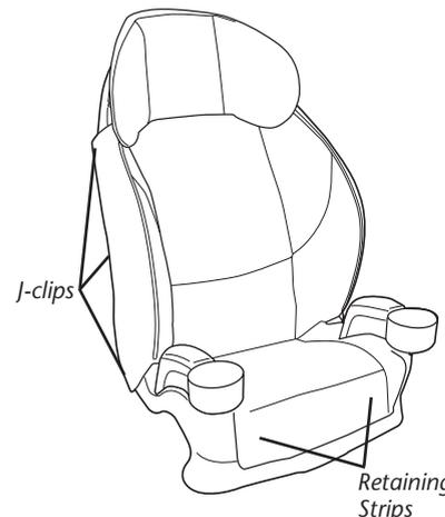
Disconnect six J-clips and two retaining strips. Remove the seat pad.
