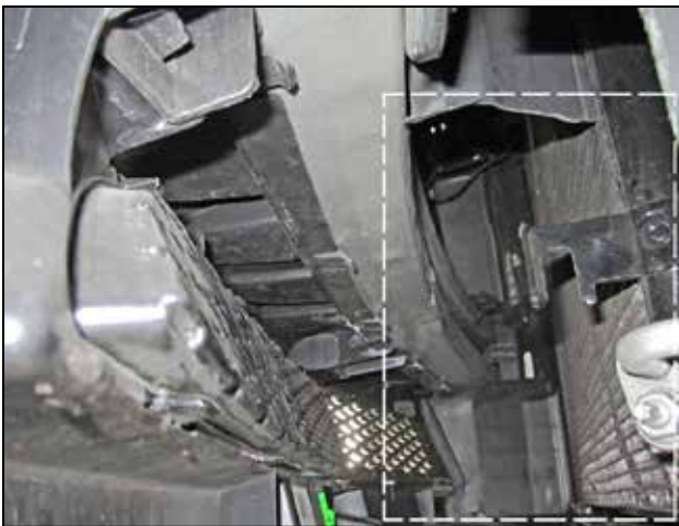
m. 2011-13 Dodge Charger Only: Front deflector after specified area is trimmed.
