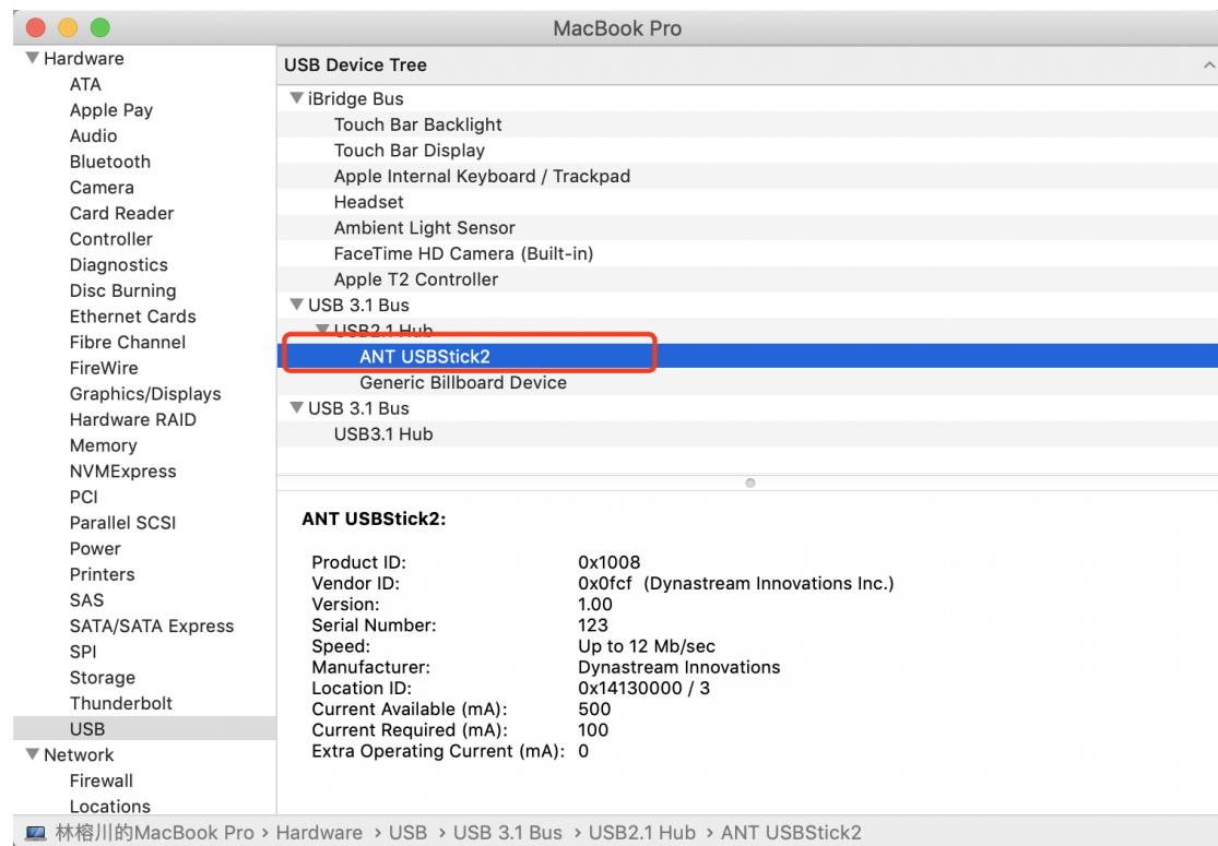
If the ANT stick is displayed in these locations, the computer recognizes that the device is connected.
