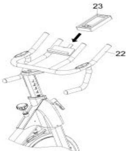
Step8.Insert the monitor on the handlebar as shown above, connect Speed cable to the counter, at last insert handle pulse sensor line to the counter.
