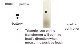
The above pictures show the wiring method for those that charging port and discharging port are the same one. If they don't share the same port, you need to make the positive of charging cable go through the hole of transformer.
