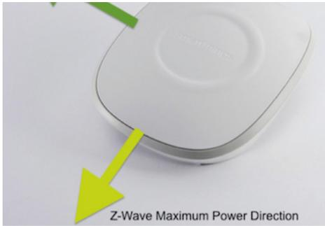
Here is a pretty good location for the Hub, in the corner of a room of the house, with the maximum power orientations pointing towards the center of the house.
