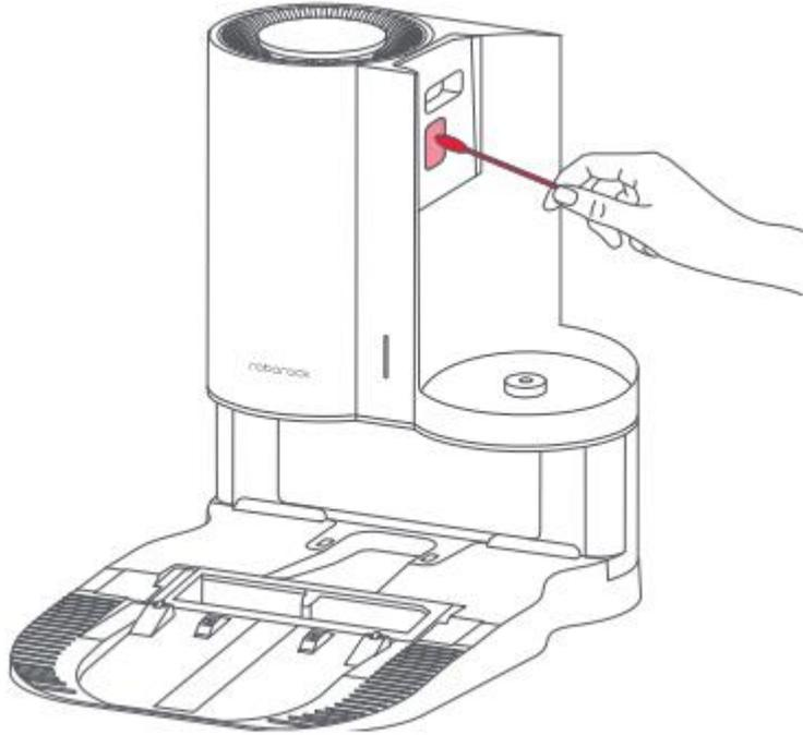
⑥ Make sure that the front filter and the rear HEPA filter are not blocked. If there is any blockage, remove and clean it.
