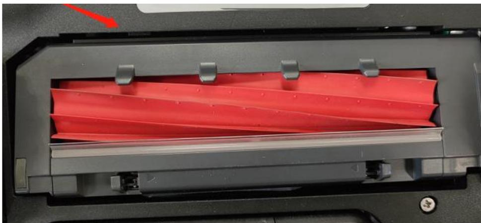
④ Remove the transparent air duct cover on the bottom of the dock and clear the blockage.
