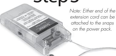
Attach the extension cord to both 'extension cord snaps' located inside the power pack.
