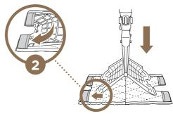
Slip the Intelli-Mop Head's 4 corner tabs into the 4 corner pockets of the Dirt Grip™ Pad.
