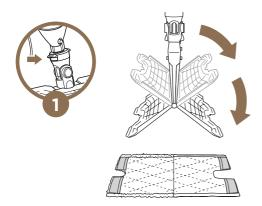
1. Lift the mop straight up by the handle until the Intelli-Mop Head is hanging straight down. Center the mop head above the pad. Press down the release buttons on the sides of the head post, and both sides of the mop head will drop open.
