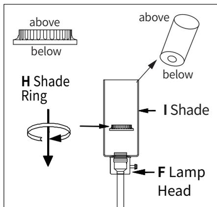
**5.** Install the prepared E26 bulb (Not included, need to be purchased separately) onto the “F Lamp Head”, and the installation is complete.
