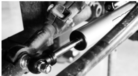
Fig. 3: Eyelet installed on track bar bolt
