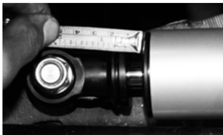
Fig. 2: 1/4" of shaft exposed
