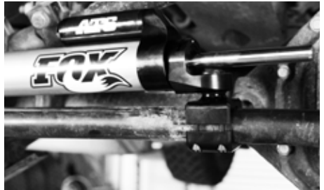
Fig. 4: Stabilizer loosely clamped to tie rod
