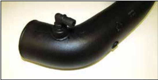
22. Install the 1/4 NPT vent fitting into the K&N® intake tube as shown.
