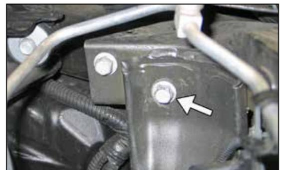
18. Remove the front fender mounting bolt shown.
