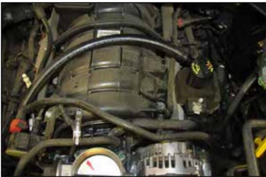
9. Install the K&N CCV hose assembly onto the factory port and position the assembly as shown.
