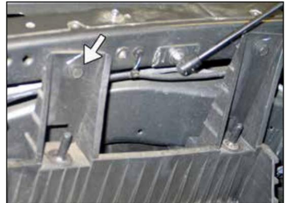
17. Remove the front air box mounting bracket bolt shown.
