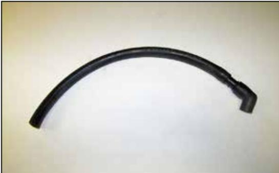
8. Remove the factory 45 deg. elbow from the factory CCV hose assembly. Assemble the K&N® CCV hose, Union and factory 45 deg. elbow as shown.
