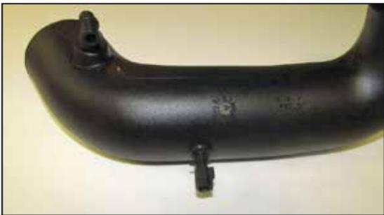
24. Install the inlet air temperature sensor into the grommet installed into the K&N® intake tube as shown.
