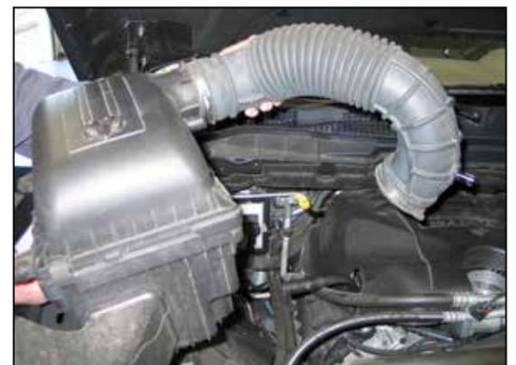
5. Disconnect the factory intake hose from the throttle body, then lift up the air box assembly and remove from the vehicle.
