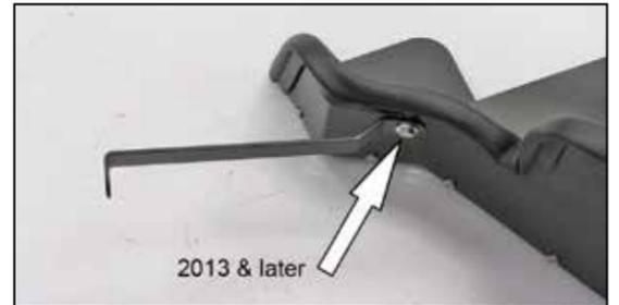
16. Install the heat shield mounting bracket (083103-1A) onto the heat shield using the provided hardware.
