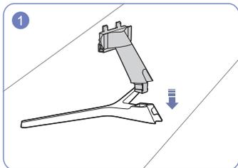
1 Insert the stand neck into the stand base in the direction shown in the figure.
