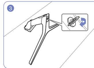
3 Tightly fasten the connecting screw at the bottom of the stand base.
