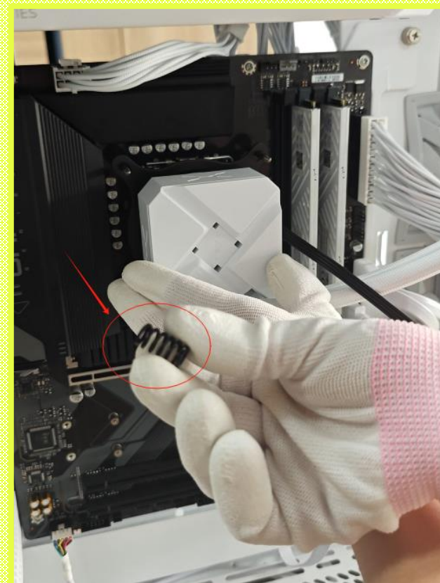
5. After locking the pump head, find the spring from the accessory bag.
